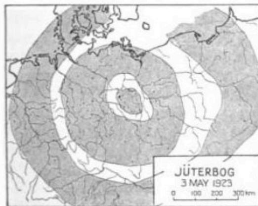
Fig. 23. Charge of 1000 kg at Jüterbog on 3 May 1923. The shaded areas show the regions of audibility.
